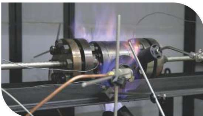
Fire Safe Testing
